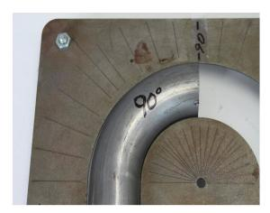
A great feature of this cutting tool is that you can drop scrap cuts into the fixture and determine what angle they were cut at. You can square up these scraps and cut them off again to a new angle to reuse them and cut waste.
