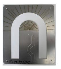
The first step is to install nuts and bolts in the four corners and center of the fixture. You want to have the fixture in about the midpoint of the bend height for easiest and most accurate marking. You can also bend the corners of the fixture to the proper height but find the nuts and bolts the easiest way to get it right.
